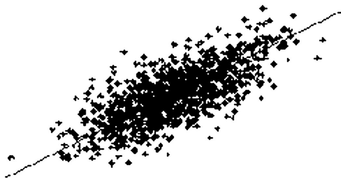
FIG. 2. Principal component analysis (PCA) of a two-dimensional data cloud. The straight line shown is the direction of the first principal component, which gives an optimal (in the mean-square sense) linear reduction of dimension from two to one.
